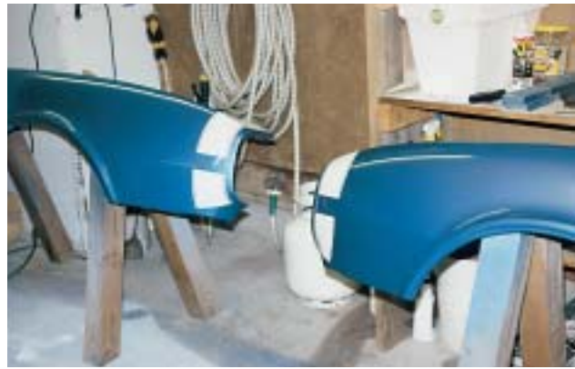
The fenders and balance panel were assembled on sawhorses. After the stripe was taped off, I disassembled the pieces and then painted the stripe.
