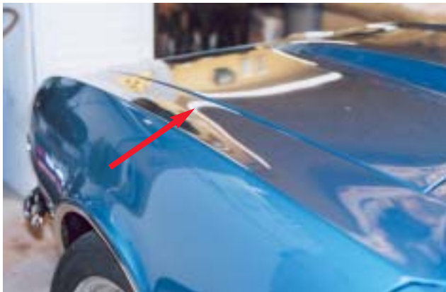
Note how the fluorescent light bends naturally with the contours.
