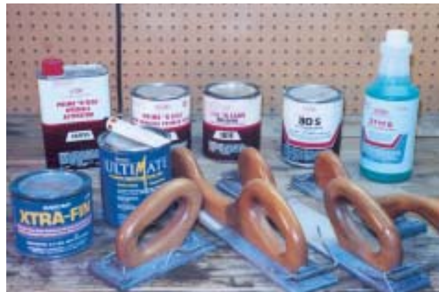
Primer, metal conditioner, bondo and sanding boards are needed for basic bodywork.
