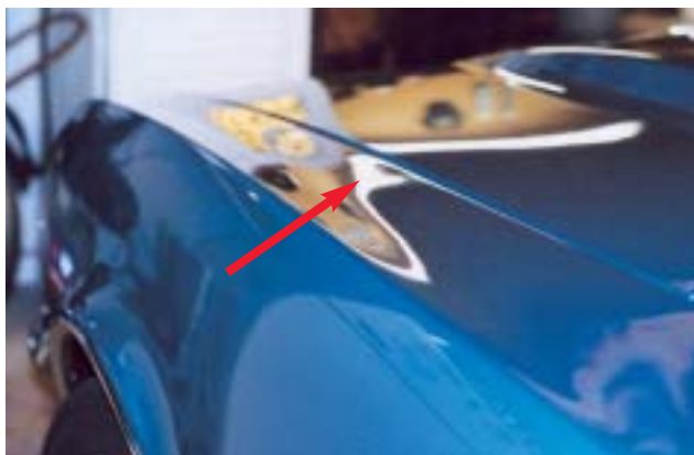
Here is a low spot I missed; notice how the light on the top fender deflects in the low spot.
